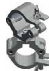
CLP-P636 weight = 1.5 kg Swivel coupler (60-63.5 mm) | SWL 650 kg (SF 8:1)
