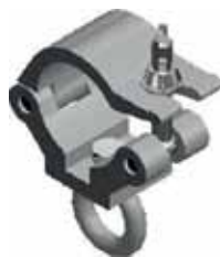
CLP-P637 weight = 1.00 kg Clamp with eye nut (60mm) | SWL 340 kg (SF 8:1)
