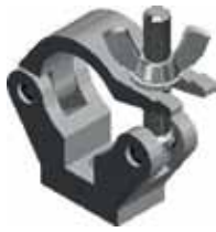
CLP-P545 ; CLP-P545B (Black) weight = 0.41 kg Clamp slim (48-51 mm) | SWL 560 kg (SF 8:1)
