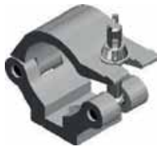
CLP-P635 weight = 0.65 kg Clamp (60 mm) | SWL 650 kg (SF 8:1)
