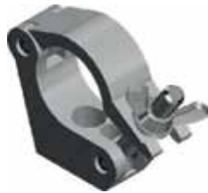
CLP-P588 weight = 0.37 kg Clamp slim side entry (48-51 mm) | SWL 410 kg (SF 8:1)
