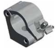
CLP-P587 weight = 0.57 kg Clamp side entry (48-51 mm) | SWL 780 kg (SF 8:1)
