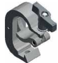
CLP-P589 ; CLP-P589B (Black) weight = 0.50 kg Clamp (48-51 mm) | SWL 350 kg (SF 8:1)
