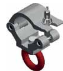
CLP-635 weight = 1.00 kg Clamp with eye nut (60mm) | SWL 650 kg (SF 8:1)
